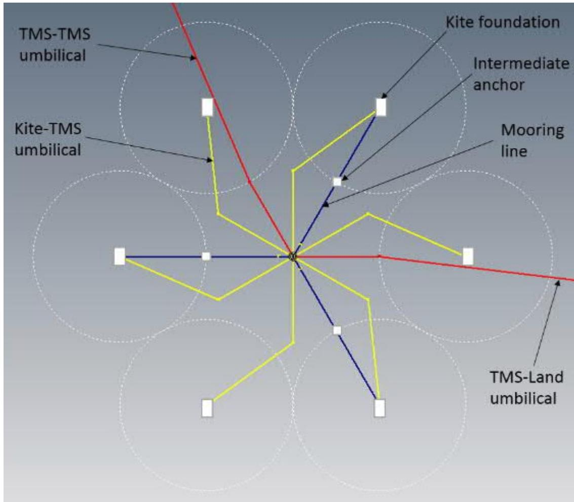
Figure 1 Kites and TMS Configuration
