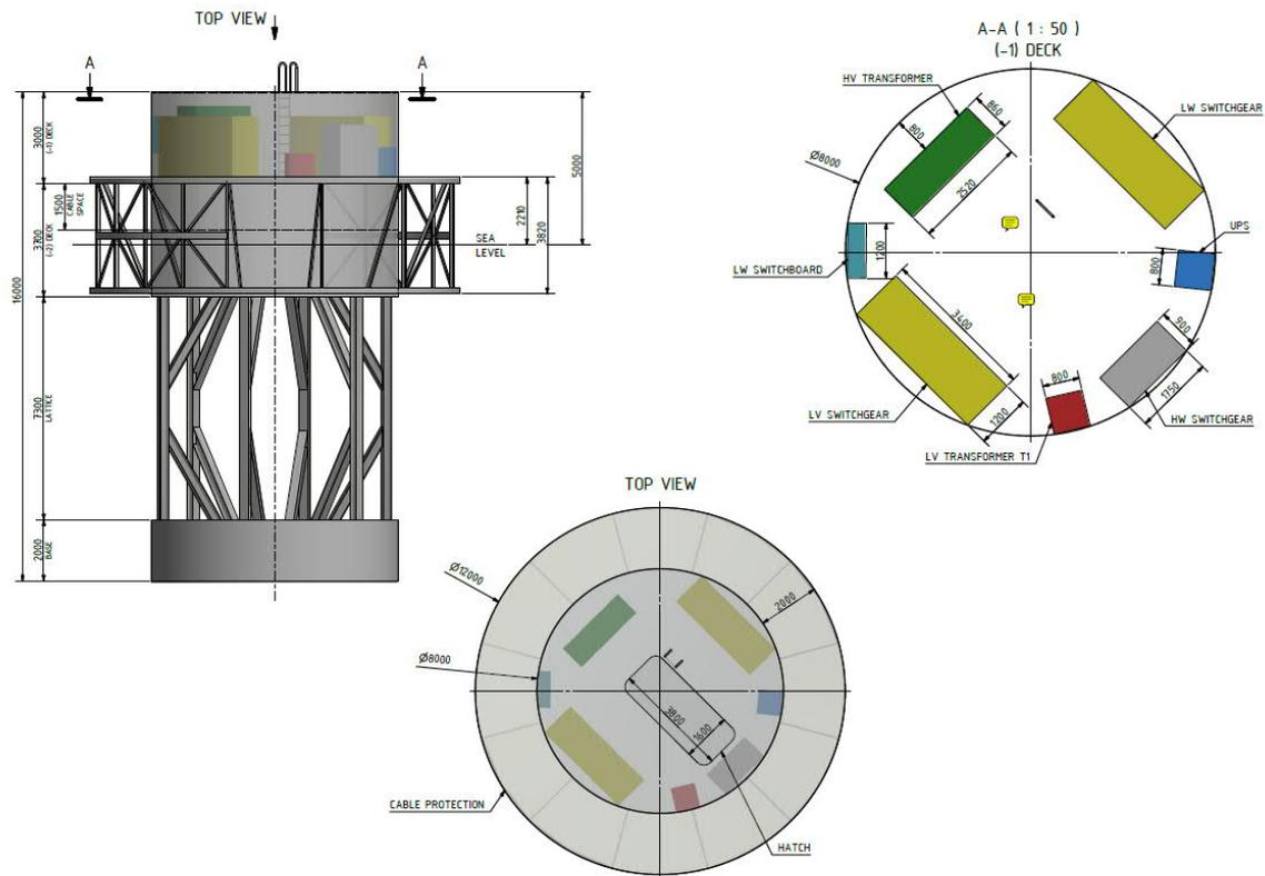
Figure 2: TMS Buoy definition
