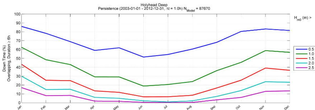
Figure 5 Holyhead Deep Annual Down Time Due to Wave Height
